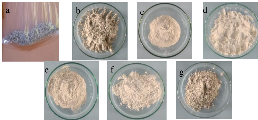
Figure 1. (a) Smaller size of Ensis sp. shell Waste, (b) uncalcined, 100 mesh, (c) calcined 900 °C, 100 mesh, (d) calcined 800 °C, 100 mesh, (e) uncalcined, 200 mesh, (f) calcined 900 °C, 200 mesh, and (g) calcined 800 °C, 200 mesh
